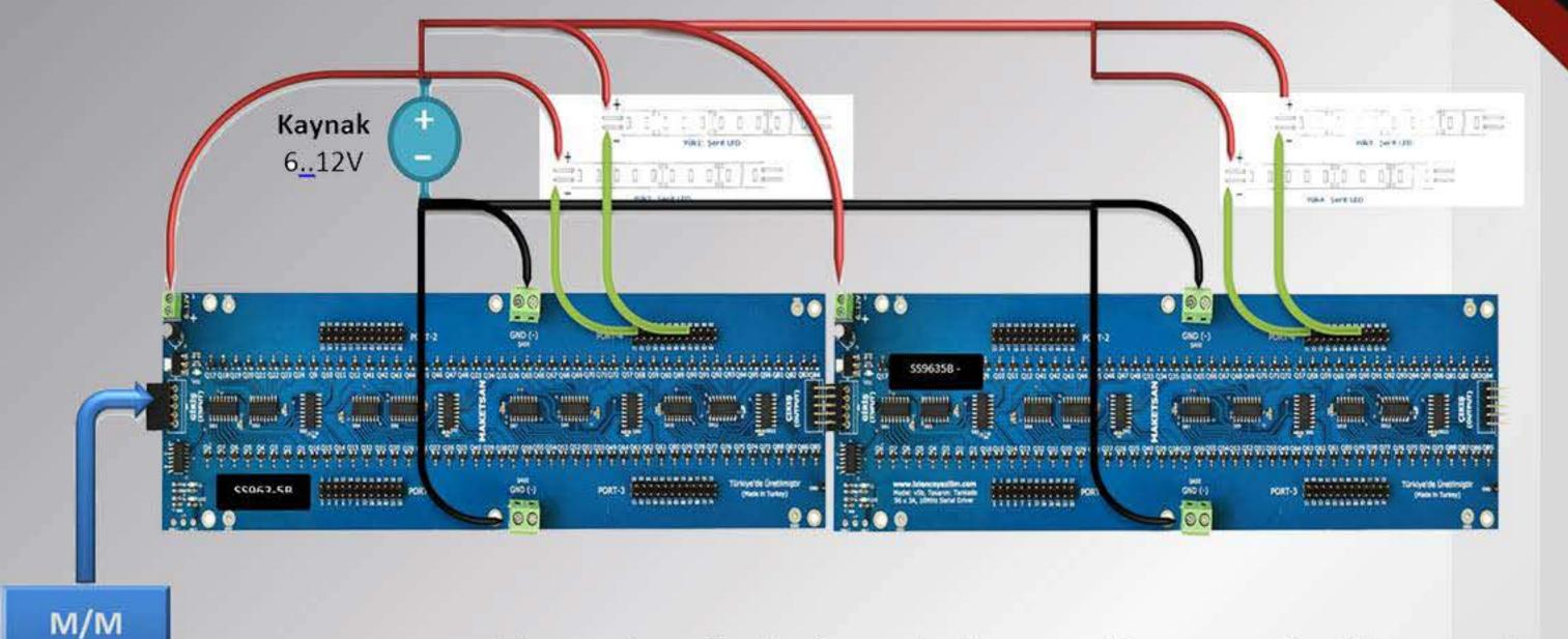
The number of outputs can be increased by connecting the cascade connection with the SS963 input and output control connectors. Up to 100 SS963 connections can be connected and controlled by
