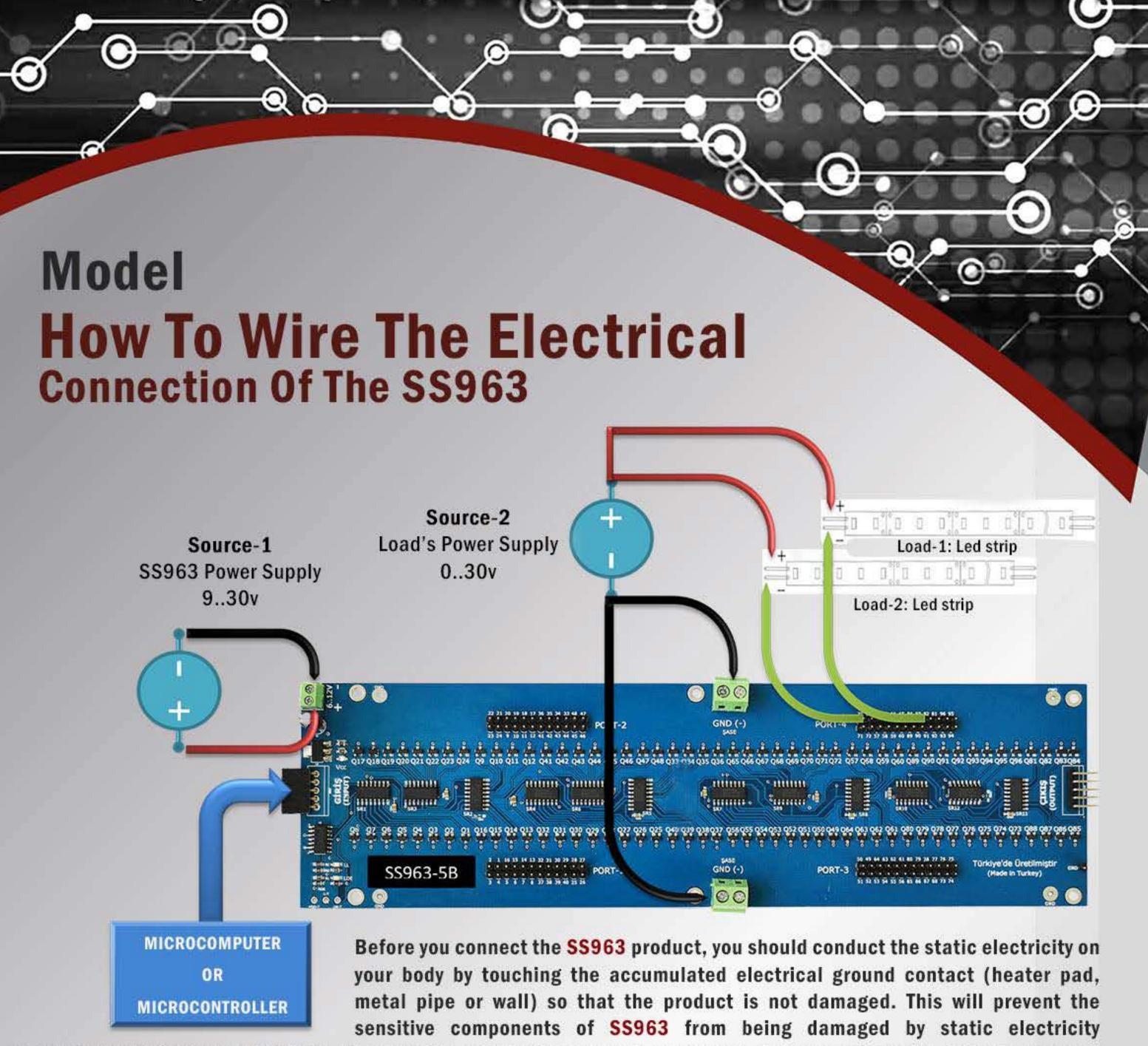
accumulated in thousands of volts. In the basic connection diagram above, two separate DC supply sources are used (Source 1 and Source 2). The sources you use must have good DC regulation. In particular, it is important that Source-1 has good DC regulation in order for \$\$\sec\$\$\$\$\$\$\$\$\$\$\$\$\$\$\$\$\$\$\$\$\$\$\$\$\$\$\$\$\$\$
